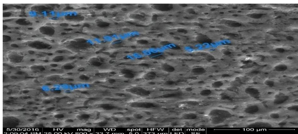
**Figure (2):** SEM image of powdered PK AC
