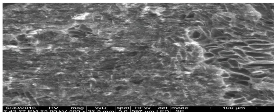
**Figure (1):** SEM image of granule PK AC
