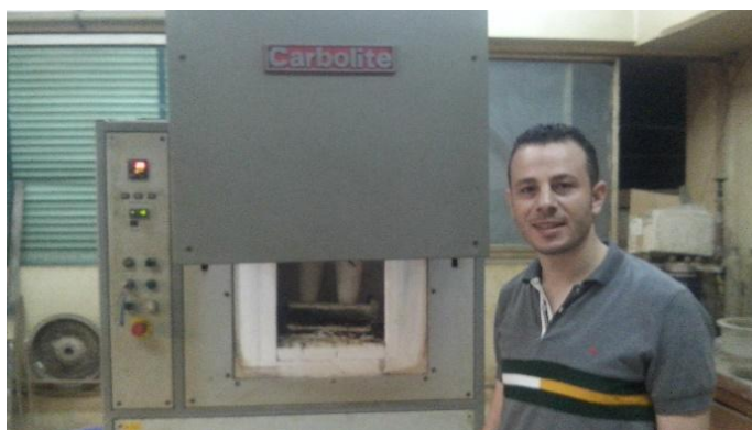
Fig. 1: The re-melting process using magnesium oxide crucible and Carbolite furnace.
