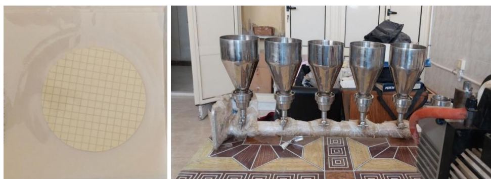
Fig.2: Filtration by 0.45µm cellulose nitrate filter paper with a vacuum system.
