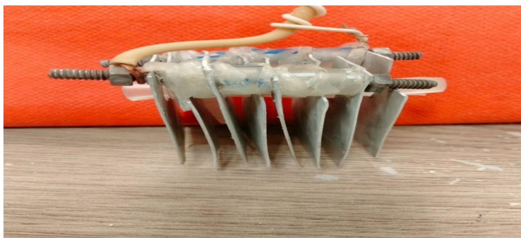
Figure 2. Electrochemical cell with aluminum plates
