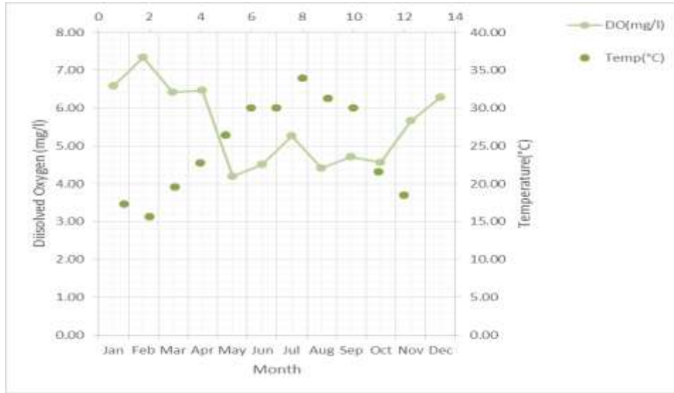
Fig. (10): Dissolved oxygen and Temperature variation in Kuwait Bay over the period from Jan to Dec.
