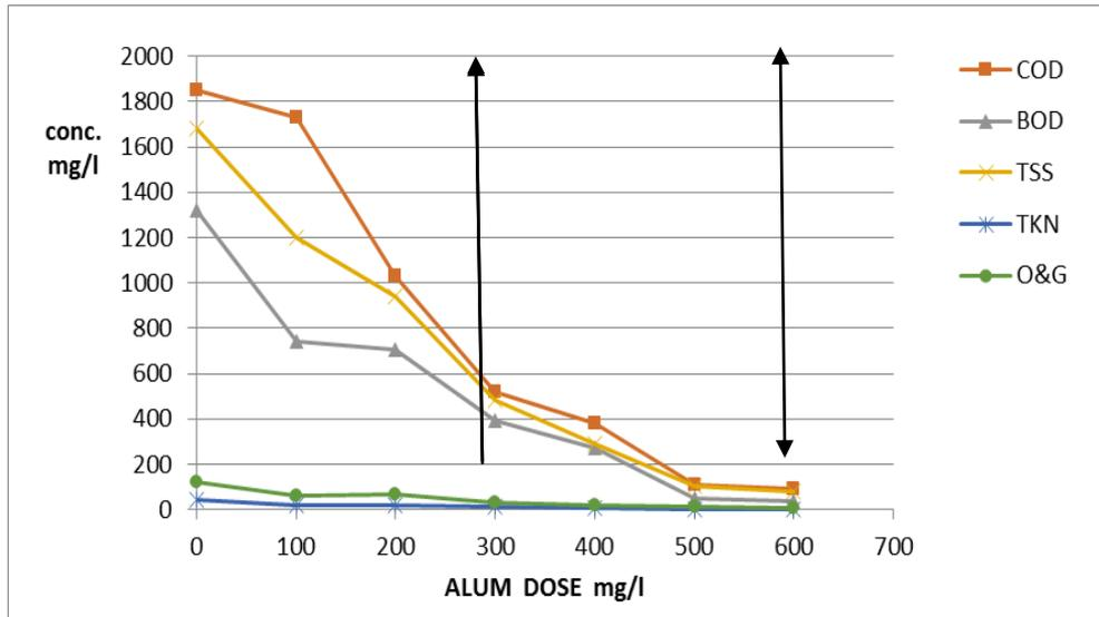
**Fig (1):** Water pollutants as a function of Alum dose (mg/l)
