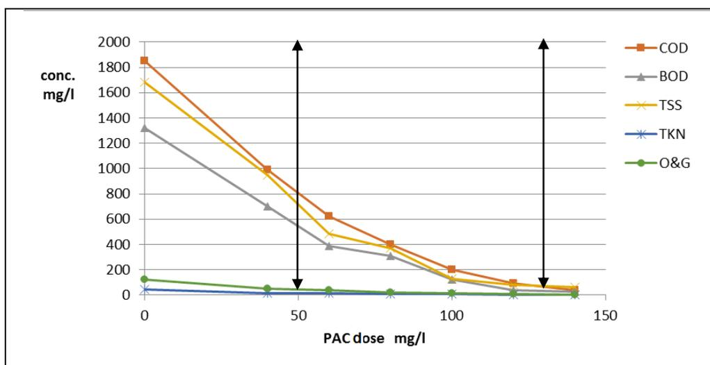
**Fig (3):** Concentration of water pollutants with PAC dose (mg/l)
