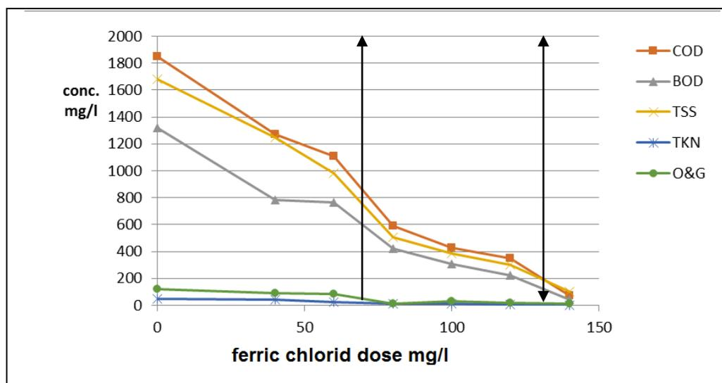
**Fig (2):** Water pollutants as a function of ferric dose (mg/l)
