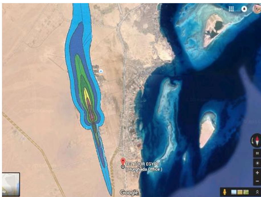
Figure (4): show the Noise prediction contour map for estimated flights For year 2027 produced by (INM) model.
