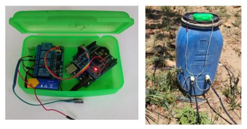
Figure (5): Suggested irrigation system control node in real system
