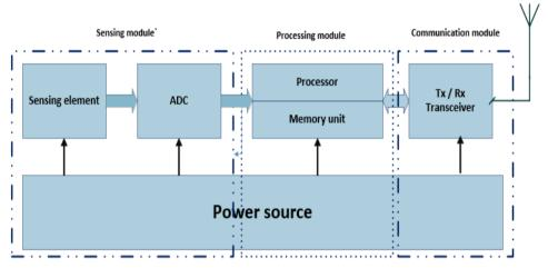
Figure (2): Sensor mote block diagram
