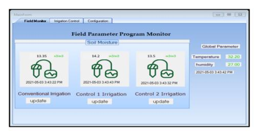
Figure (8): Field monitor tab form to monitor the field parameters soil moisture, temperature, and humidity.
