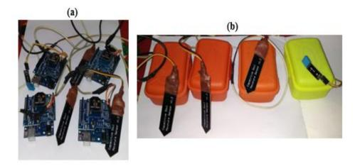
Figure (6): Real picture (a) sensor mote (b) sensor mote in plastic case
