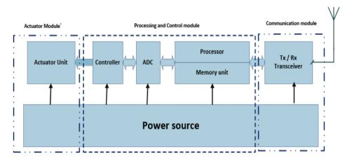
Figure (3): Actuator mote block diagram
