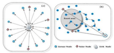
Figure (4): (a) Sink Based WSAN Topology,(b) Multi Hop Sink Based WSAN
