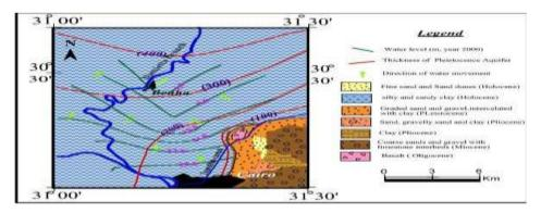
Fig(4): Flow lines of groundwater, the Quaternary aquifer, East Cairo area, Egypt (modified after RIGW 1992; Geriesh *et al.*, 2008).
