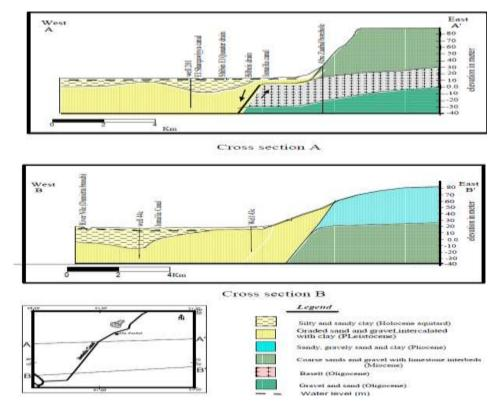
Fig(3): Hydrogeological cross sections at different locations (After RIGW, 1989).
