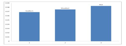
Figure 2: Mean concentrations of Total dioxin and furan compound (PCDD's and PCDF's) of incinerators
