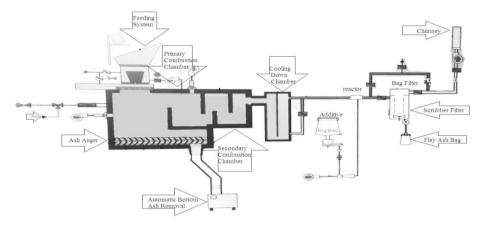
Figure 1: Components of incinerator
