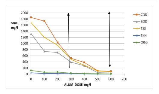
Fig (1): Water pollutants as a function of Alum dose (mg/l)
